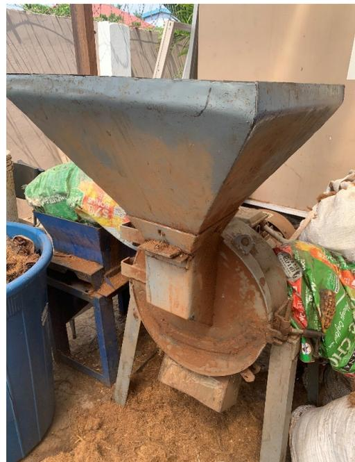
Figure 10. Hammer Mill Machine
