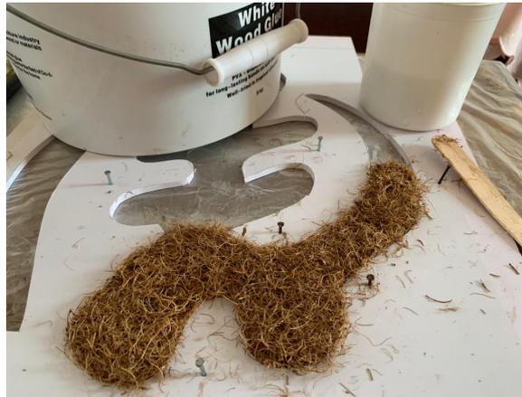
Figure 16. Stuffing the fibres into the adinkra mould
