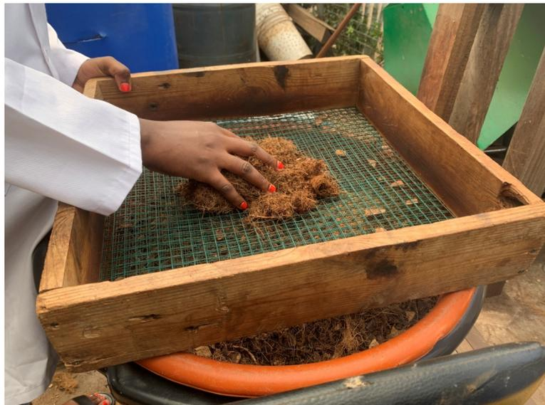
Figure 12. Sieving the Grinded Husks
