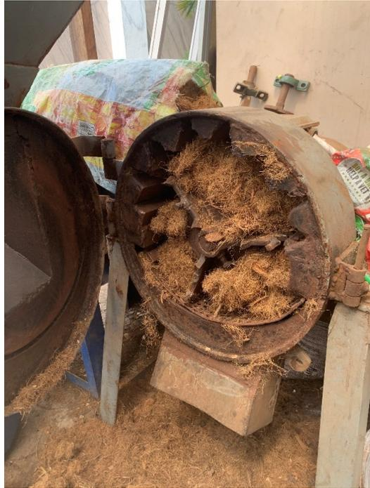
Figure 13. Grinded Husk in the Hammer Mill Machine
