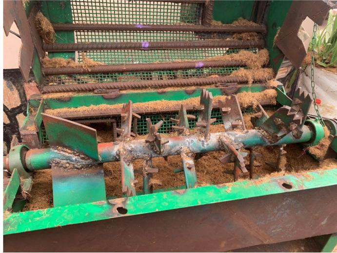
Figure 11. A Grinding machine that was built by Kmoy Cocopeat Company
